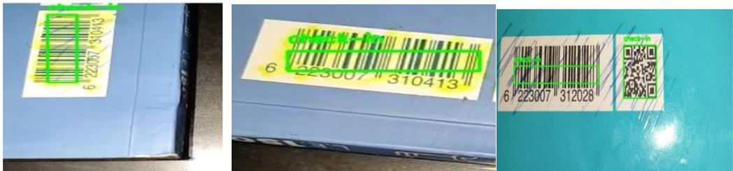
**Fig. 17. Capturing a distorted one-dimensional and two-dimensional barcode in the dark with a pen and colors using the mobile flash**
