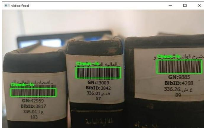
**Fig. 6 The process of borrowing three books together at the same time**
