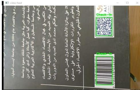
**Fig. 9. Capturing one- and two-dimensional barcodes**
