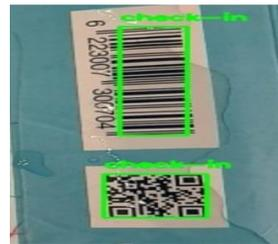
**Fig. 19. Capturing a one- and two-dimensional barcode with a layer of water on it**
