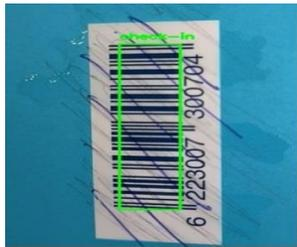
**Fig. 18. Capturing a distorted one- and two-dimensional barcode with a pen with a layer of water on it**
